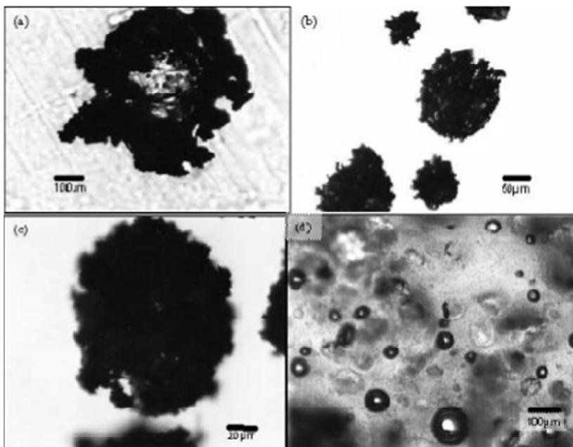
Figure 2: The SEM images of microcapsules incorporated PU.
