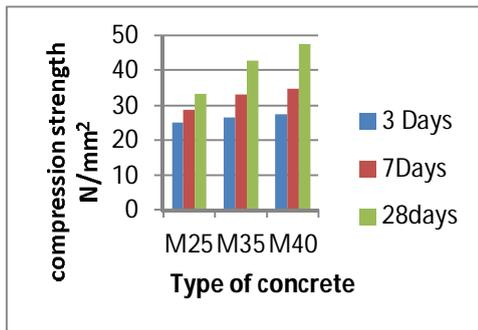
Fig.7 Conventional concrete
