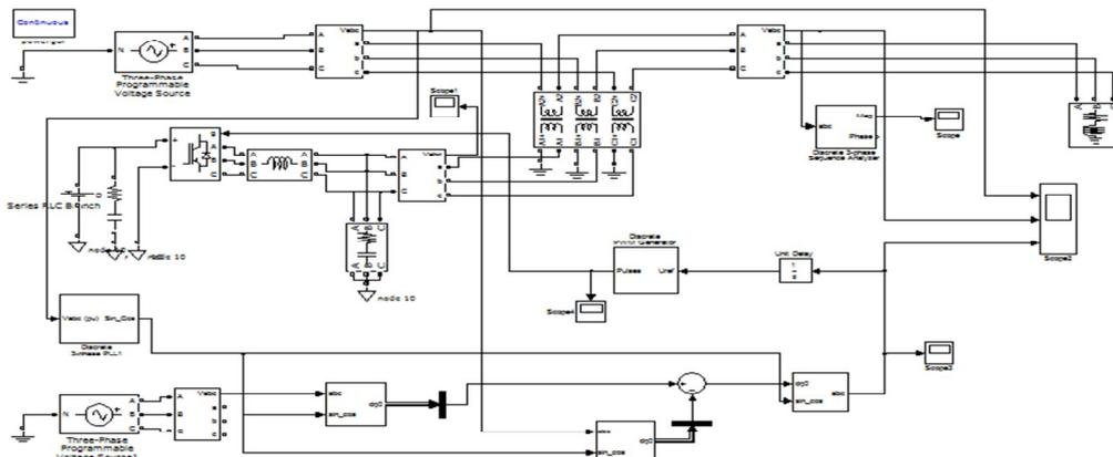
Figure-5:MATLAB model of DVR connected system
