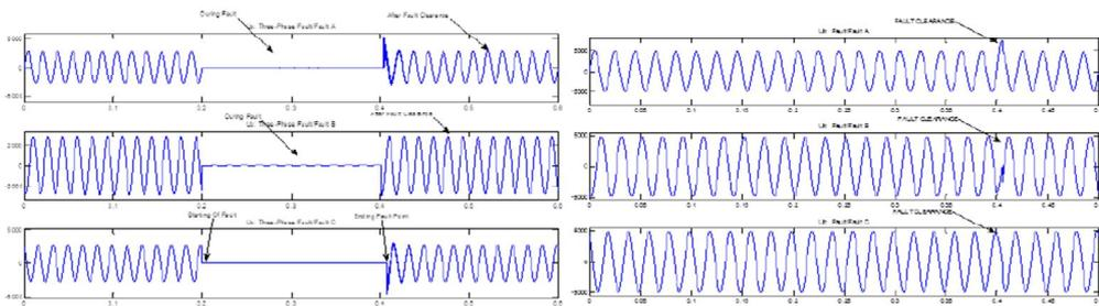
Fig.-8(a) Three phase fault without DVR Fig.-8 Three phase fault with DVR voltage compensation
