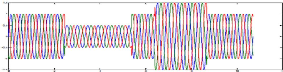
Fig.-7(a) Supply Side Voltage with 50% voltage Sag and 50% voltage Swell
