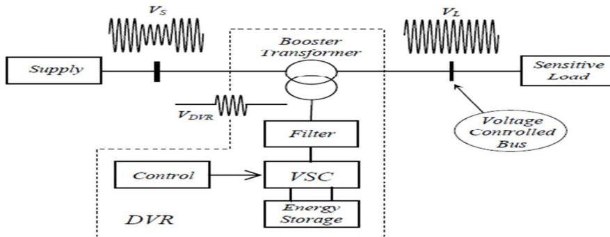
Figure-1: DVR series connected topology
