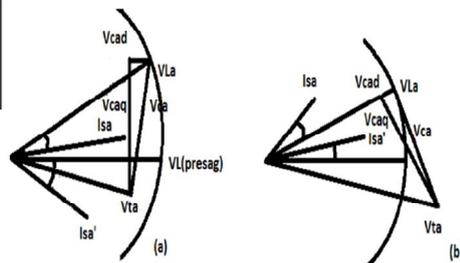
Figure-2 (a) Schematic diagram of DVR Figure-3: Phasor Diagram for (a) Voltage Sag (b) Voltage Swell
