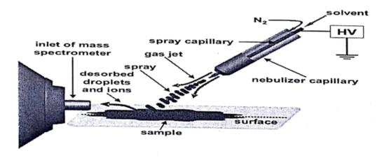
In this method analyte particals are solvated by an ionized solvent flow, the mechanism and spectra are very much similar to ESI. This can be used in Pharmaceutical testing like QC/QA, Counterfeit identification, Chemical weapons and latent fingure prints.
